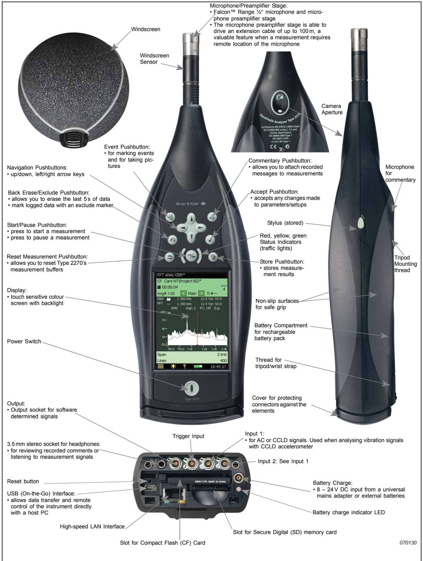
Fig. 4 Key features of Hand-held Analyzer Type 2270
