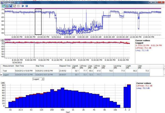
**TEST EQUIPMENT:** B&K 2270 Analyzer SN 2644661 + B&K 4193 Microphone SN 2643922 **CALIBRATION:** Factory 10/3/11 – verified immediately prior to test **TIMING & FREQUENCY WEIGHTING SETUP:** Fast response / A + C weighting **PROCEDURE:** monitoring / logging of noise at typical location on site **PRIMARY NOISE SOURCE:** HVAC units during normal operation **PRESENT:** R. Lemker
